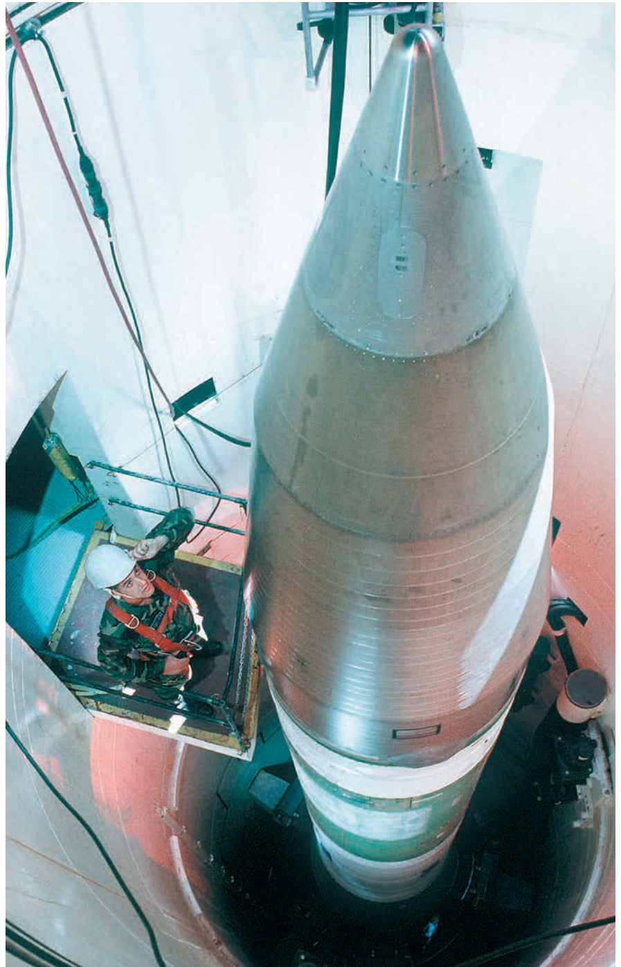
SSgt. Stephen Kravitsky inspects a Minuteman III missile inside a silo near Grand Forks AFB, N.D., in 1989.
