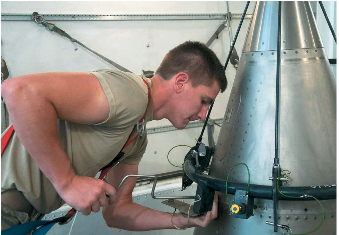
A1C William Ray removes the screws holding the Minuteman III nose point to the rest of the re-entry system while aboard a payload transporter in the F.E. Warren AFB, Wyo., missile complex in 2016.
