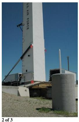
The downstage of the Minuteman III missile located at this launch facility near Brady, Mont. is lifted into the transporter-erector July 12. This mission completed the first missile removal and marked the start of Defense Department-directed deactivation activities in the 564th Missile Squadron at Malmstrom Air Force Base, Mo
